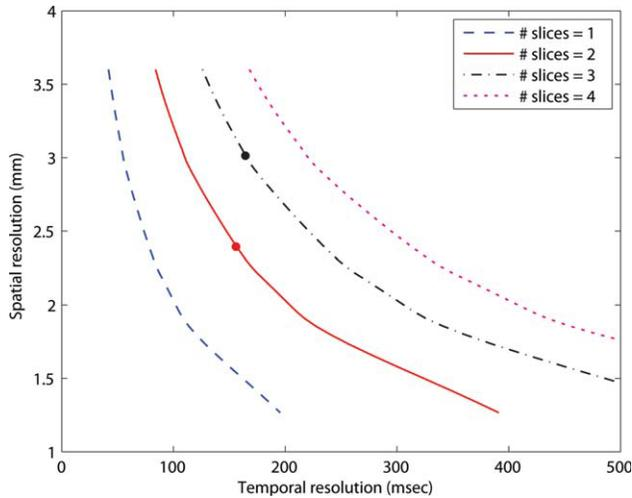
**Figure 2.** Spatial-temporal resolution trade-off. Interleaved spiral trajectories were designed with a field-of-view (FOV) of 20 cm and readout duration of approximately 2.5 ms. Spatial and temporal resolutions indicated by the red and black dots were used for time-interleaved imaging of 2 and 3 slices, respectively. [Color figure can be viewed in the online issue, which is available at [wileyonlinelibrary.com](http://wileyonlinelibrary.com).]
